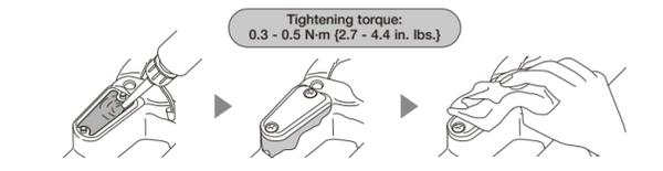
7. Return the brake lever to its original position.
