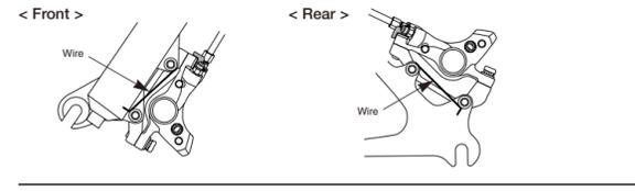
For C-shaped guides and the usual type of cable stoppers, use the special Shimano cable supporter (sold separately) to secure as shown in the illustration.
