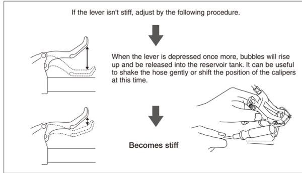
5. With the brake lever depressed, open and close the bleed nipple in rapid succession (for approximately 0.5 seconds each time) to release any air bubbles which may be in the calipers. Repeat this procedure about 2 to 3 times. Then tighten the bleed nipple again.
