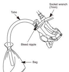
3. Loosen the bleed nipple by 1/8th of a turn to open it, and then pour oil into the reservoir tank. Gently operate the brake lever while doing this to help prime the system with the oil.
