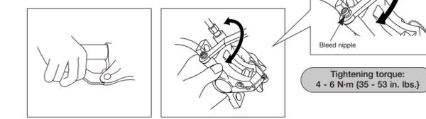
6. Fill the reservoir tank with oil and then replace the reservoir tank cover. Fill the reservoir tank to overflowing with oil while replacing the cover to ensure that no air bubbles remain inside the reservoir tank. In addition, be careful not to get any oil on parts such as the rotor and brake pads.
