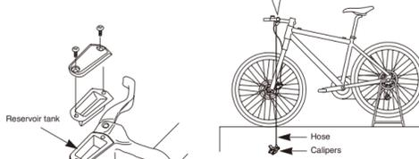
2. Set a 7mm socket wrench in place, attach a bag to the tube, and then place the tube onto the bleed nipple as shown in the illustration.
